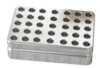
35-well for 1.5 ~ 2.0mL conical centrifuge tube or 1.0mL cryogenic vial.
