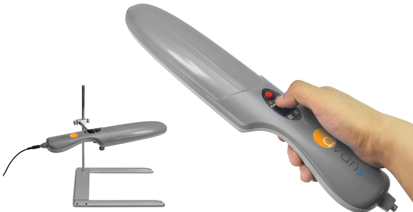
AgileUV™ portable UV detector provides optional single wavelength 365nm and 254nm, or double wavelengths 365nm / 254nm. It is used for detection of nucleic acid dye, such as Ethidium bromide, Acridine orange, in fluorescence dyes. It is widely used for nucleic acid testing in many industries including molecular biology, biological chemistry, medical science, forensic autopsy examination as well as biological agent.
